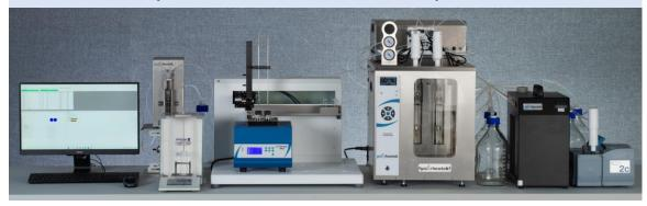
RPV Auto Polymer Viscometer System with - integrated sample preparation, single zone reaction block (heating, stirring, and cooling), Rheotek Smart Sampler, RPV Gen 3 viscometer with two measuring positions, optional diaphragm vacuum pump
