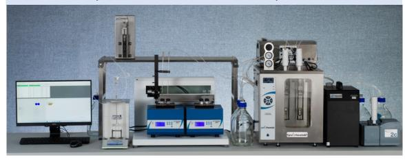
RPV Auto Polymer Viscometer System with – integrated sample preparation, dual zone reaction blocks (heating, stirring, and cooling), Rheotek Smart Sampler, RPV Gen 3 viscometer with two measuring positions, optional diaphragm vacuum pump and shelf.
