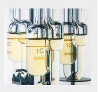
The RPV Auto Polymer Viscometer uses glass capillary tubes blown in-house and calibrated by the PSL ISO17025 accredited laboratory.
