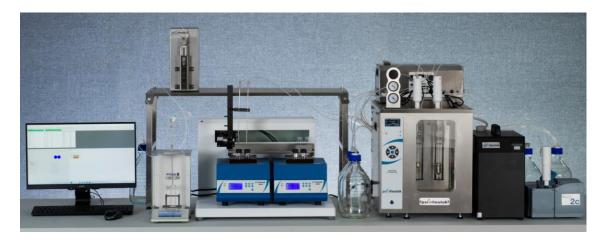
RPV fully Automated Polymer Viscometer System – including integrated sample preparation, sample dissolution, sample loading, temperature control, flow time measurement, reporting of results and in-situ cleaning and drying.
